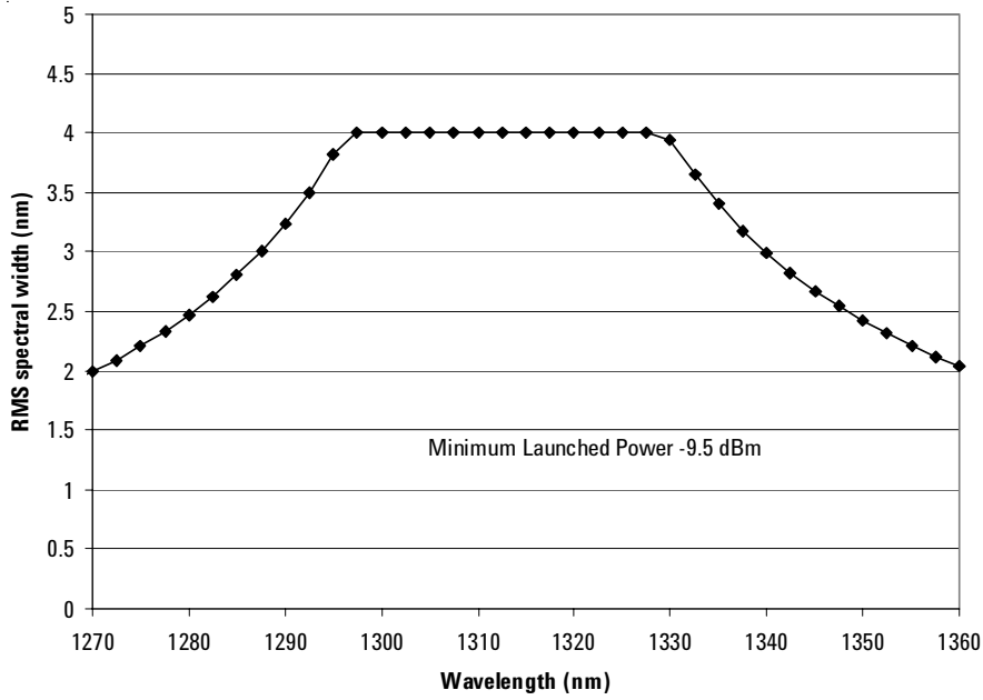
Figure 10. Maximum spectral width trade off curve derived from Gigabit Ethernet link model
